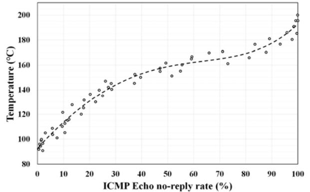
Fig. 9. Relation between ICMP Echo no-reply rate and the furnace temperature.
