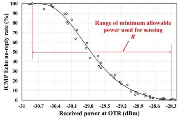
Fig. 3. Relation between the received power and the ICMP Echo no-reply rate.
