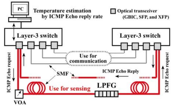
Fig. 1. Temperature-sensing system employing OTRs and an LPFG.
