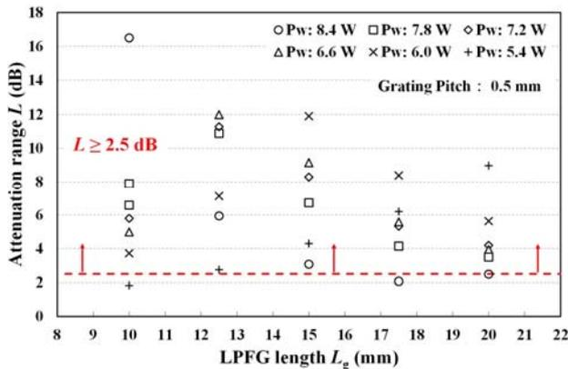
Fig. 5. Attenuation ranges of the attenuation band in the loss spectra of the fabricated LPFGs.
