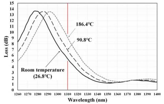
Fig. 7. Temperature dependence of the shift in the LPFG optical loss spectrum.
