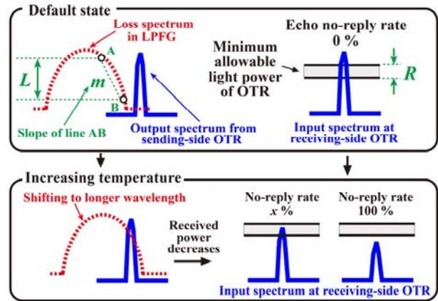
Fig. 2. Mechanism of temperature sensing.
