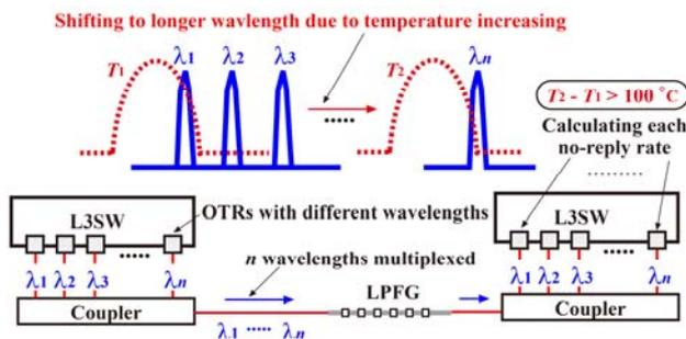
Fig. 10. Measurable temperature range expanded by  $n$  OTRs.
