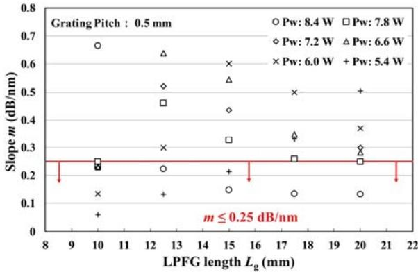
Fig. 4. Slope of the attenuation band in the loss spectra of the fabricated LPFGs.
