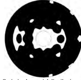
Fig. 2. Optimized material distribution of ferrite material (black) for Example 1
