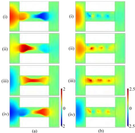
Fig 7. Electric fields of optimized configuration: (a) Example 1 at 2.0 GHz; (b) Example 2 at 3.25 GHz for various phases of incident waves: (i)  $0^\circ$ ; (ii)  $60^\circ$ ; (iii)  $120^\circ$ ; (iv)  $180^\circ$ .
