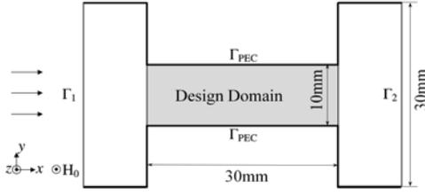
Fig 1. Design domain and boundary conditions.
