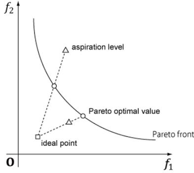
Fig. 4. Pareto optimal solution when searching by STOM
