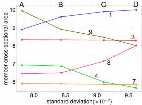
Fig. 10. Transitions of member cross-sectional areas for designs A, B, C, and D
