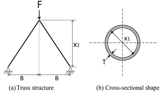
Fig. 5. Two-bar truss design problem
