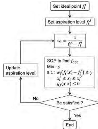
Fig. 3. Computational flow of STOM
