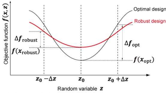
Fig. 1. Concept of robust optimization
