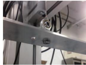
(a) Rod end connecting tie cable and rib
