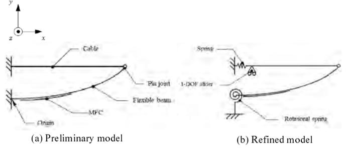
Fig. 5 Boundary conditions of finite-element (FE) models.
