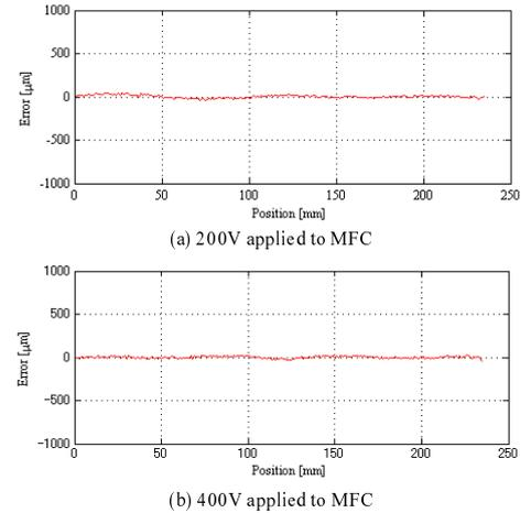
Fig. 9 Difference between experiment and FE analysis after FE-model updating with MFC actuation.
