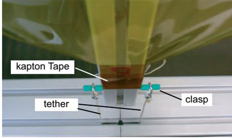
Fig. 3 Bottom corner fixed to frame.
