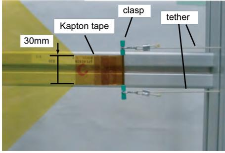
Fig. 2 Corner stiffened by polyimide tape.
