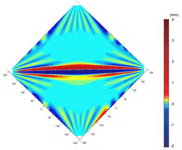
Fig. 12 Wrinkle distribution obtained by FEM analysis
