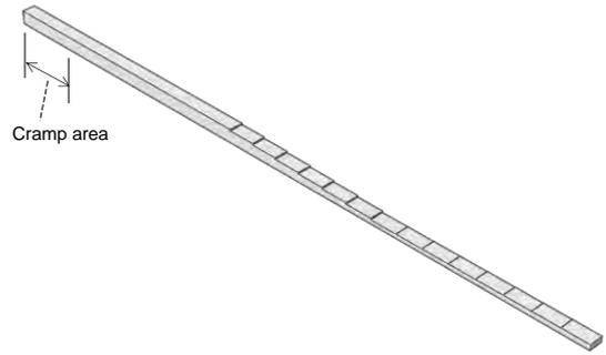
Fig. 9. Rib configuration obtained by optimization
