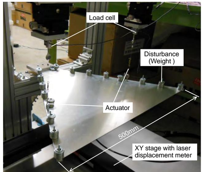
Fig. 10. Experimental setup
