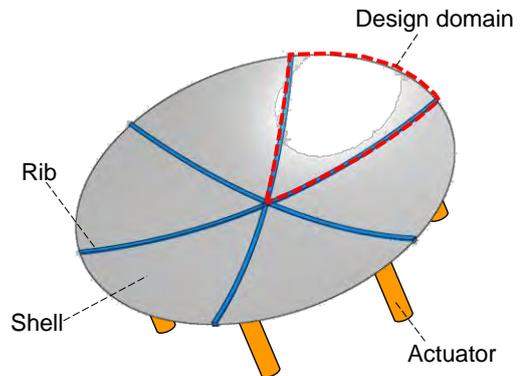
Fig. 1. Overview of rib-stiffened shell antenna
