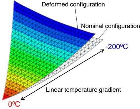
Fig. 4. Deformed configuration of nominal design under disturbance without shape correction
