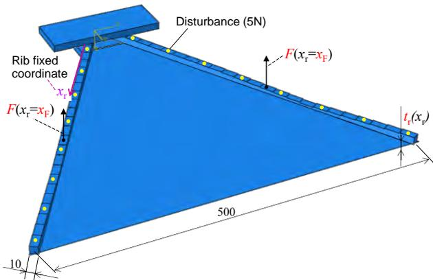
Fig. 7. Analysis model of flat rib-stiffened shell antenna
