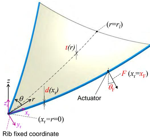
Fig. 2. Analysis model of rib-stiffened shell antenna
