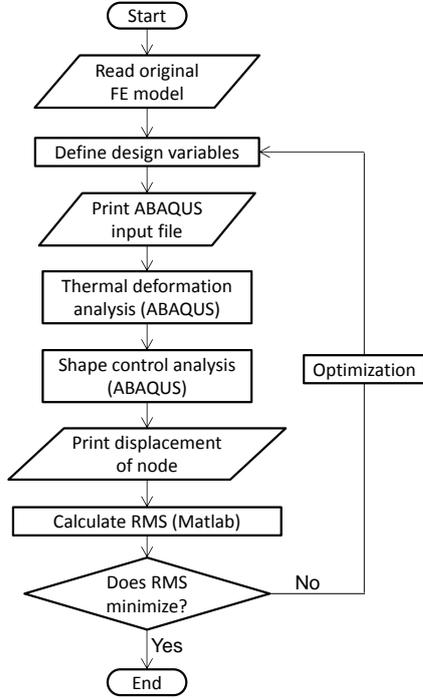
Fig. 3. Flowchart of design optimization process
