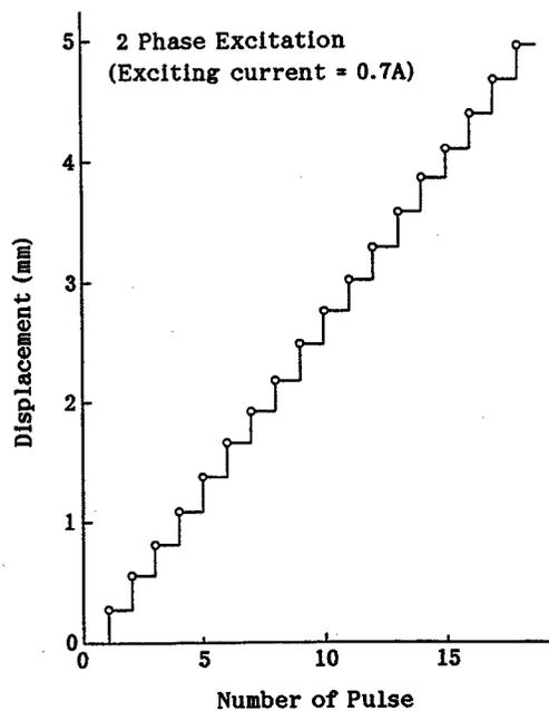
Fig. 4 Pulse-displacement characteristics.
