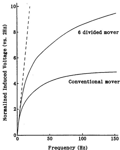
Fig. 8 Electromagnetic effect of the 6 divided mover.
