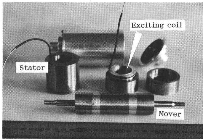
Fig. 1 Components of the cylindrical linear pulse motor.
