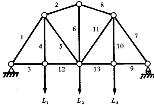
Fig. 5. Thirteen member statically determinate truss
